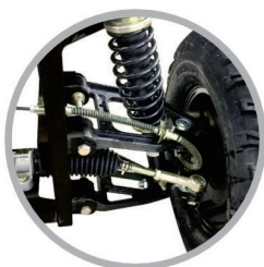
双叉臂独立悬架 Independent Front Suspension with Double Swing Arm
